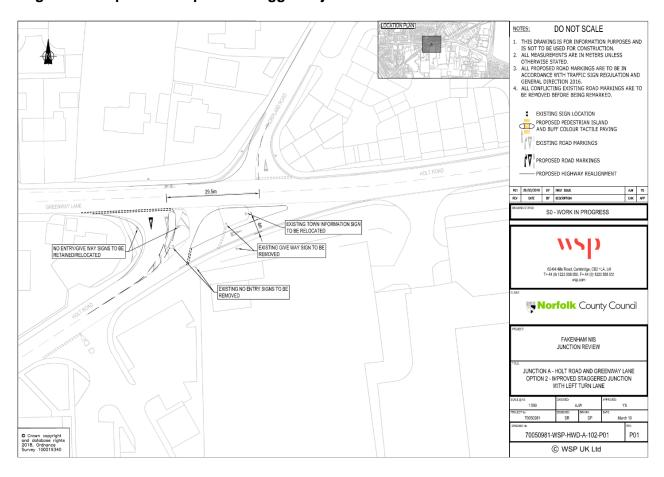
This option has a similar layout to the existing junction and operationally should perform the same way as the existing layout. For this reason, this option has not been modelled. However, this improvement should bring some benefits for Non-Motorised Users to cross the junction as the junctions will be slightly smaller, as shown in Appendix 2.
