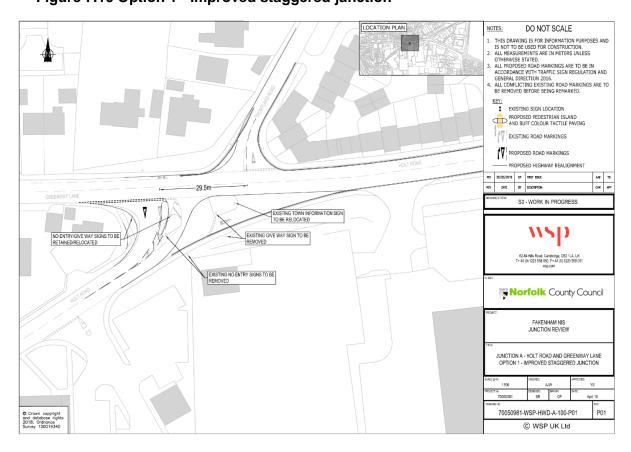
This improvement considers removing the segregated left turn southbound lane, realigning kerbs and introducing a new splitter island on the Holt Road south approach to the junction, as shown in Appendix 2. This junction improvement should bring more opportunities for improving NMUs facilities. The main benefits of this option are:
