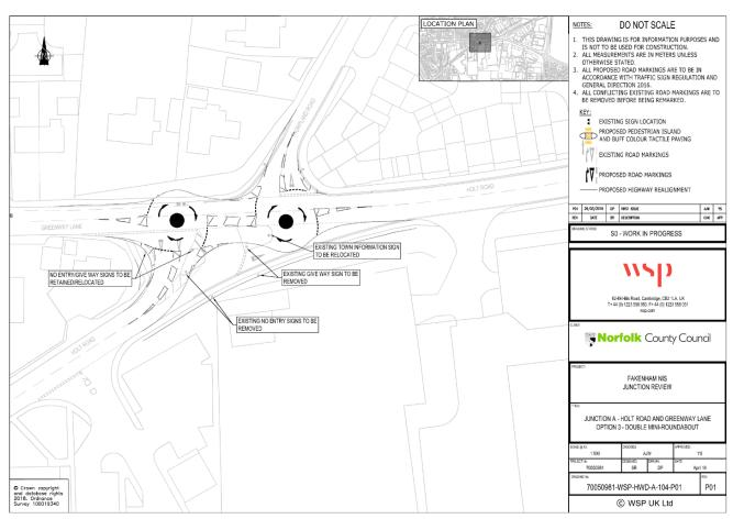
This improvement is the most intrusive option and consists of a complete junction resign to include double mini roundabouts, as shown in Appendix 2. The double mini roundabout design will act as a traffic calming measure. This should provide a safer environment for NMUs.
