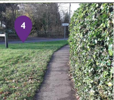
The hedge is encroaching on to the footpath, reducing the path width to 90cm on the approach to the road crossing at Skeyton New Road
