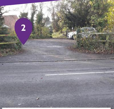
There is a 20mm step out of the car park and on to the footpath where the surface changes to paved concrete
