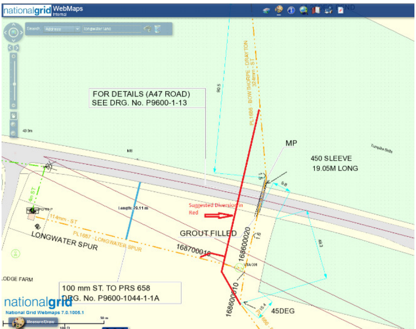
Figure 8.1 Suggested Diversion in red (approx. 100m). Note this will potentially include a 324mm and 114mm tee and three way stopples and bypass
