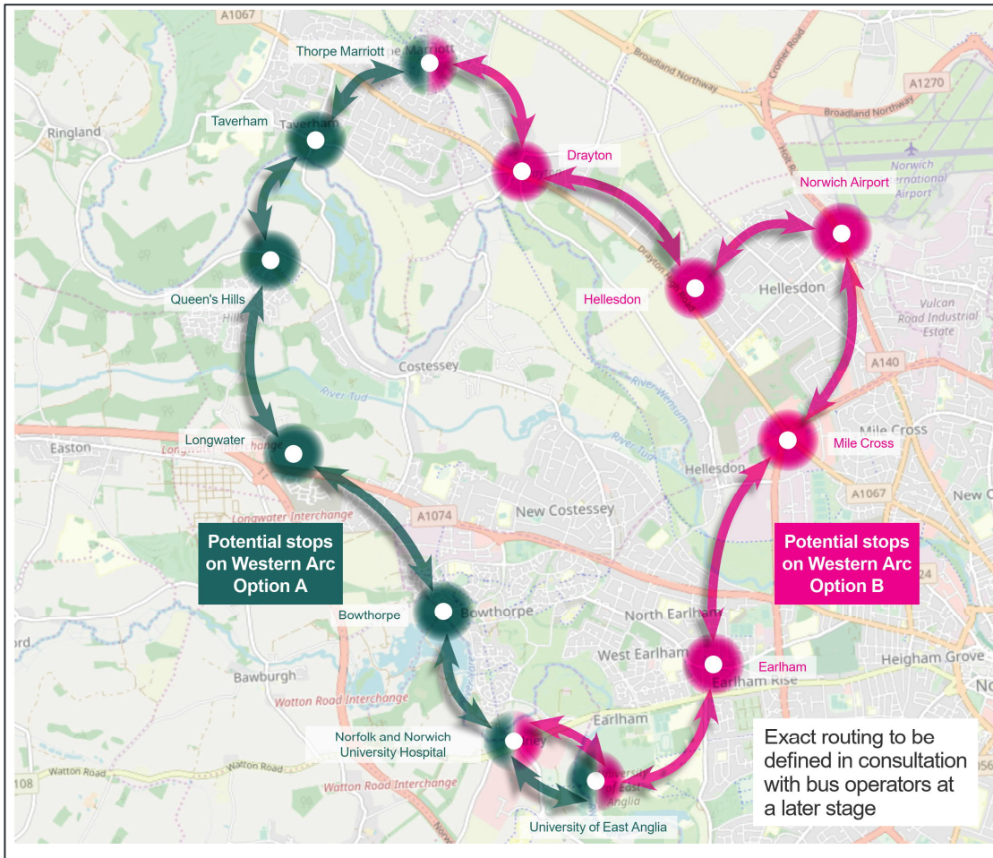
Figure 7-6 - Proposed Western Arc Service route alignment
