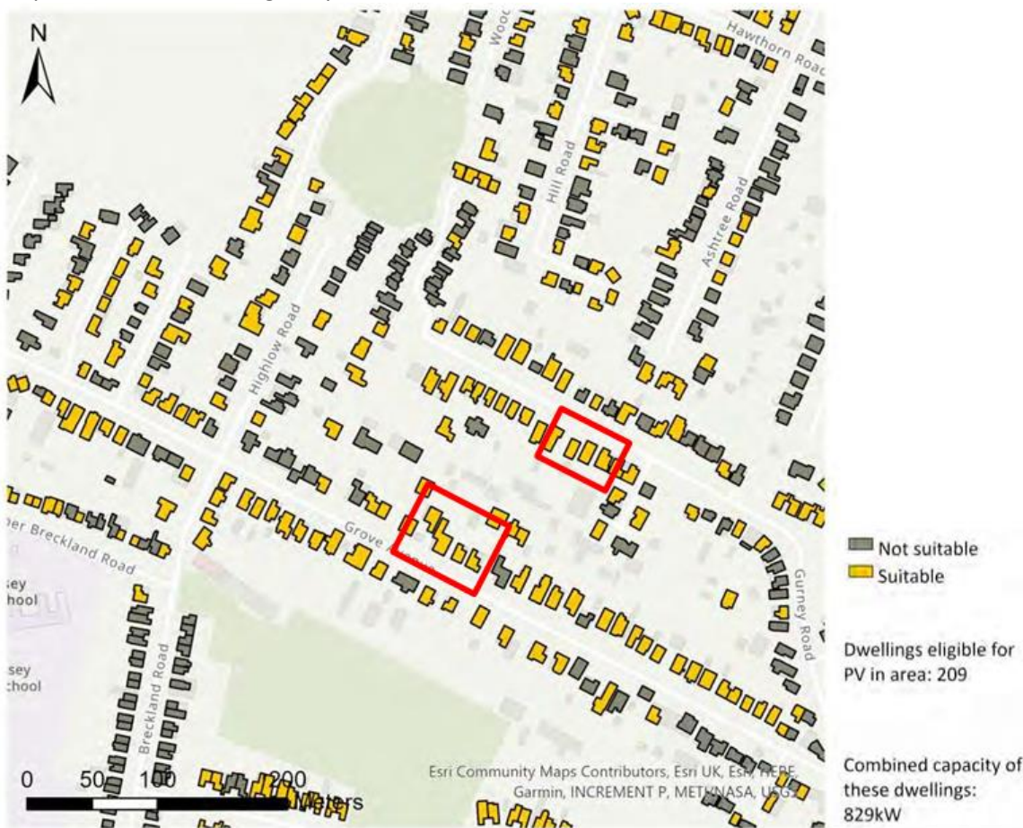
Figure 103: Dwellings identified as suitable for rooftop PV panels. (Location: New Costessey, Norwich )
