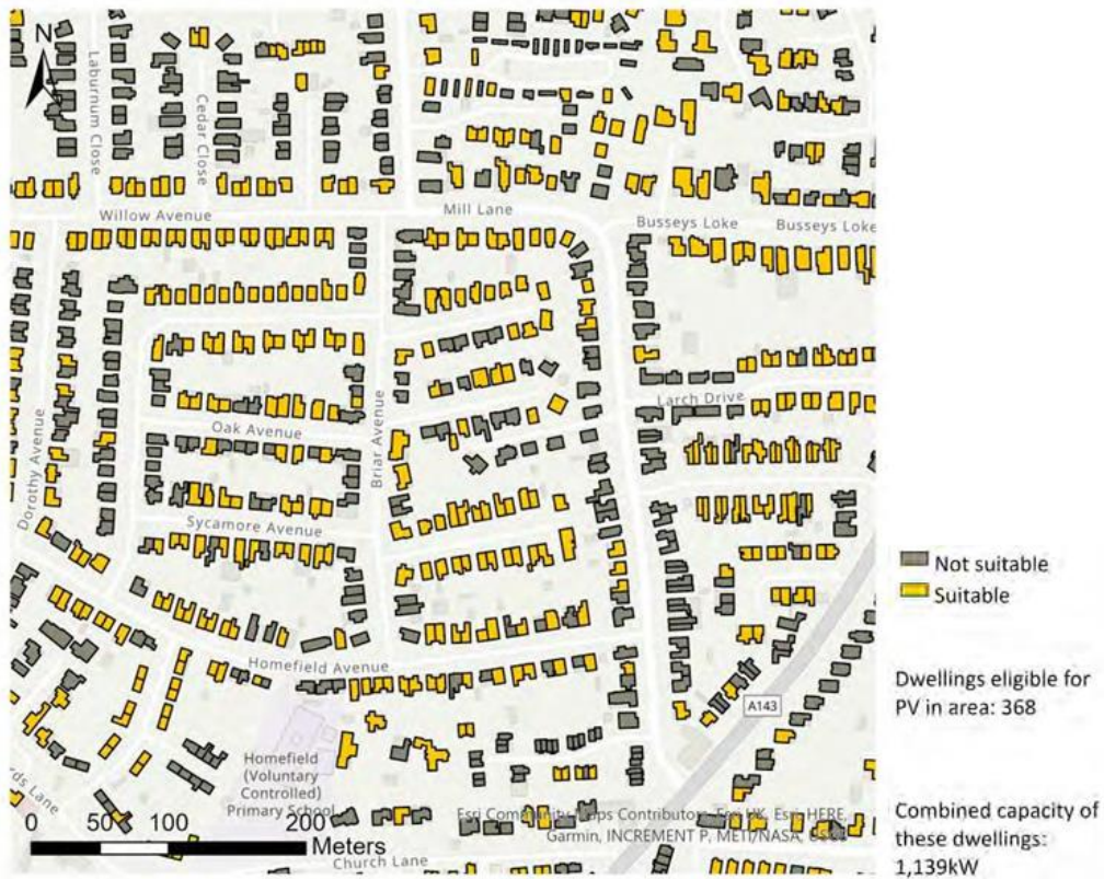
Figure 93: Dwellings identified as suitable for rooftop PV panels. (Location: Bradwell, Great Yarmouth )
