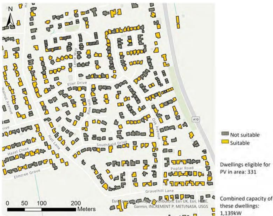
Figure 28: Dwellings identified as suitable for rooftop PV panels. (Location: West Winch, King's Lynn )
