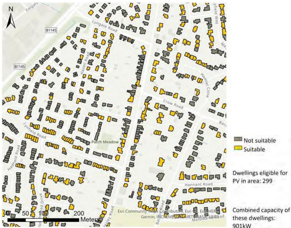
Figure 95: Dwellings identified as suitable for rooftop PV panels. (Location: Patch Meadow, North Walsham )
