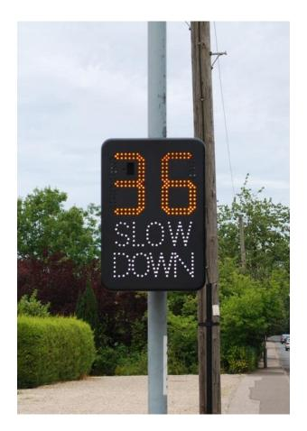
Our Speed Indicator Device with Slow Down (SAM 2) shows the speed of oncoming vehicles and has a variety of different settings to show a different display when speeds are either above or below the speed limit.
