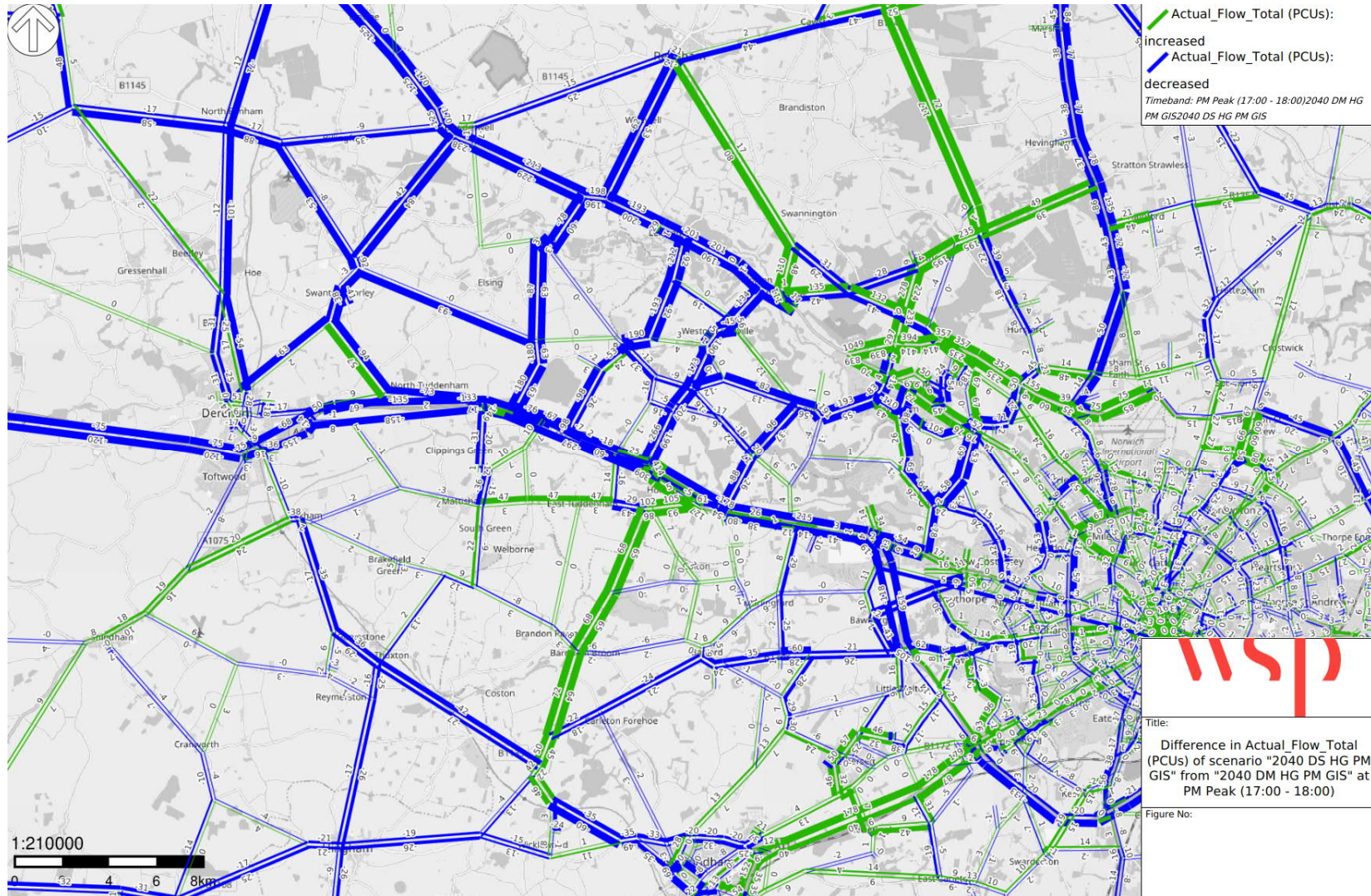
Figure 11-11: 2040 High Growth DS scenario versus 2040 High Growth DM scenario, Actual Flow Difference, in pcu's - PM peak
