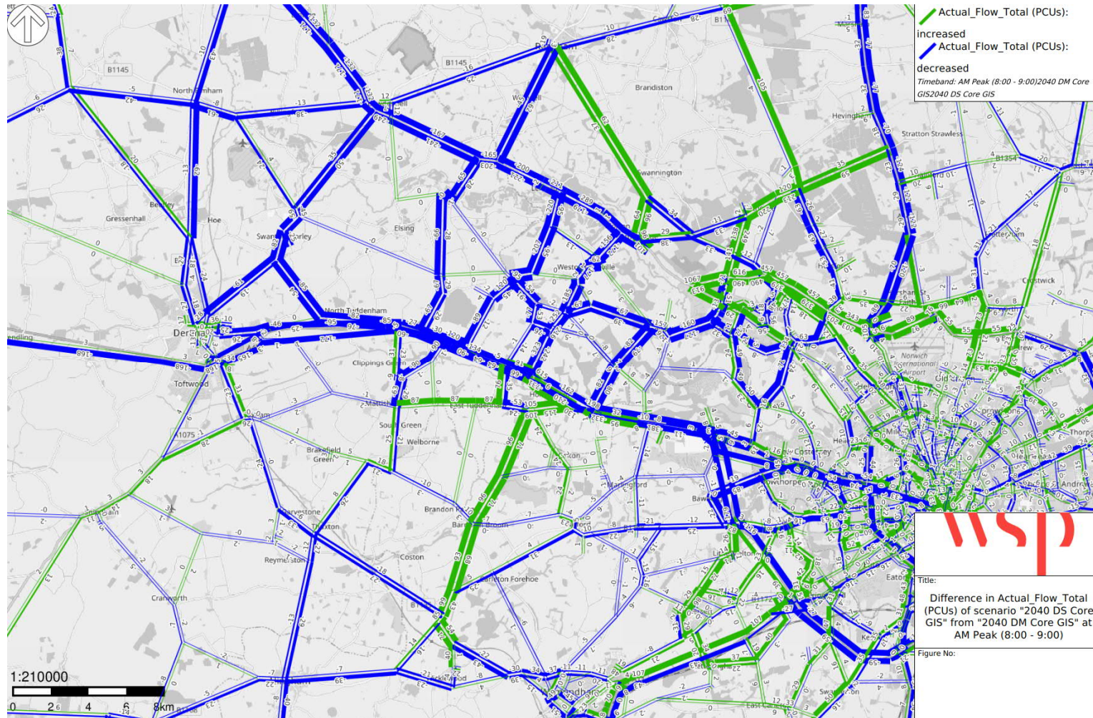
Figure 9-7: 2040 Core Growth DS scenario versus 2040 Core Growth DM scenario, Actual Flow Difference, in pcu's - AM peak
