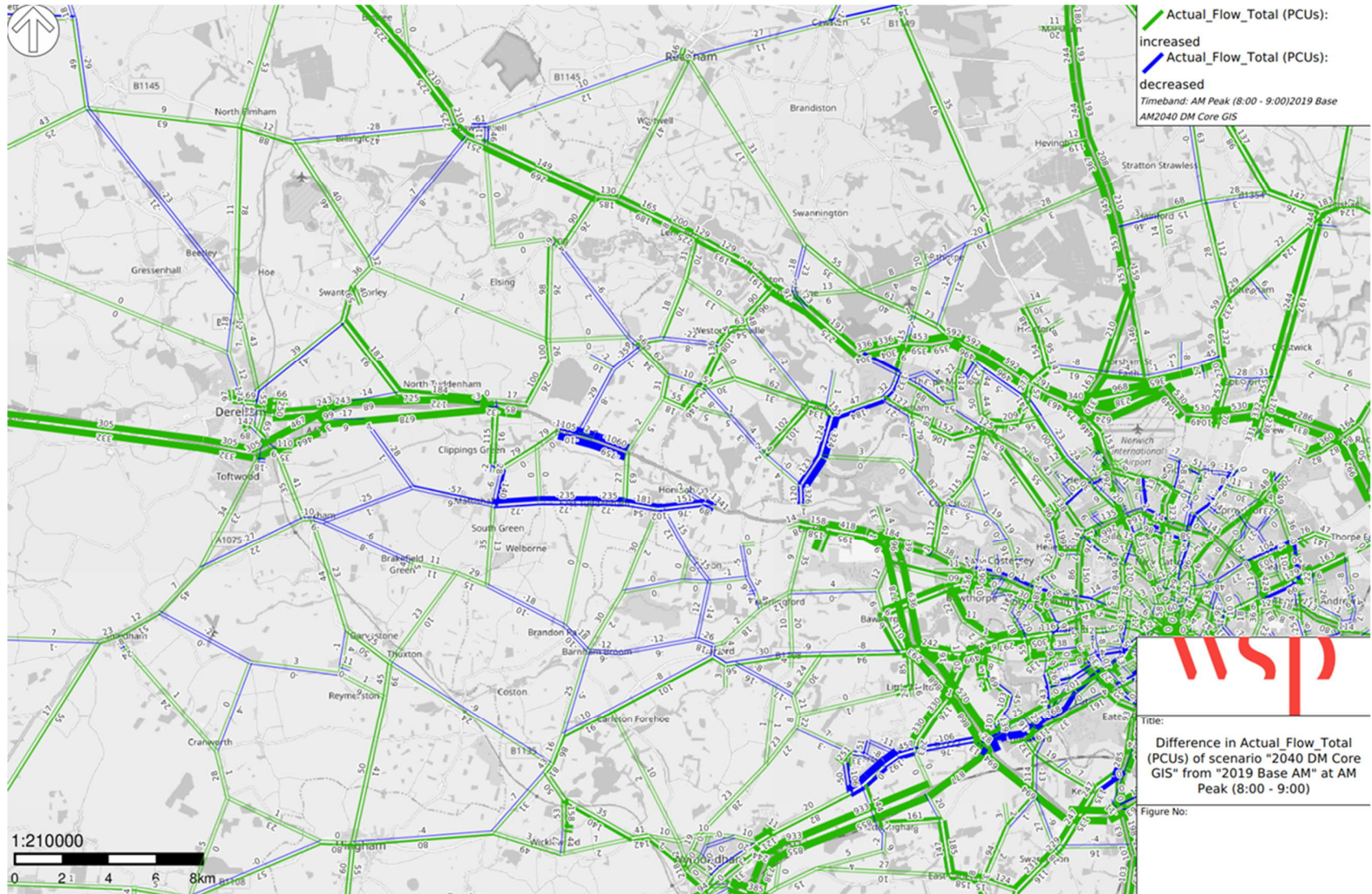
Figure 9-1: 2040 Core Growth scenario versus 2019 Base Year model, Actual Flow Difference, in pcu's - AM peak
