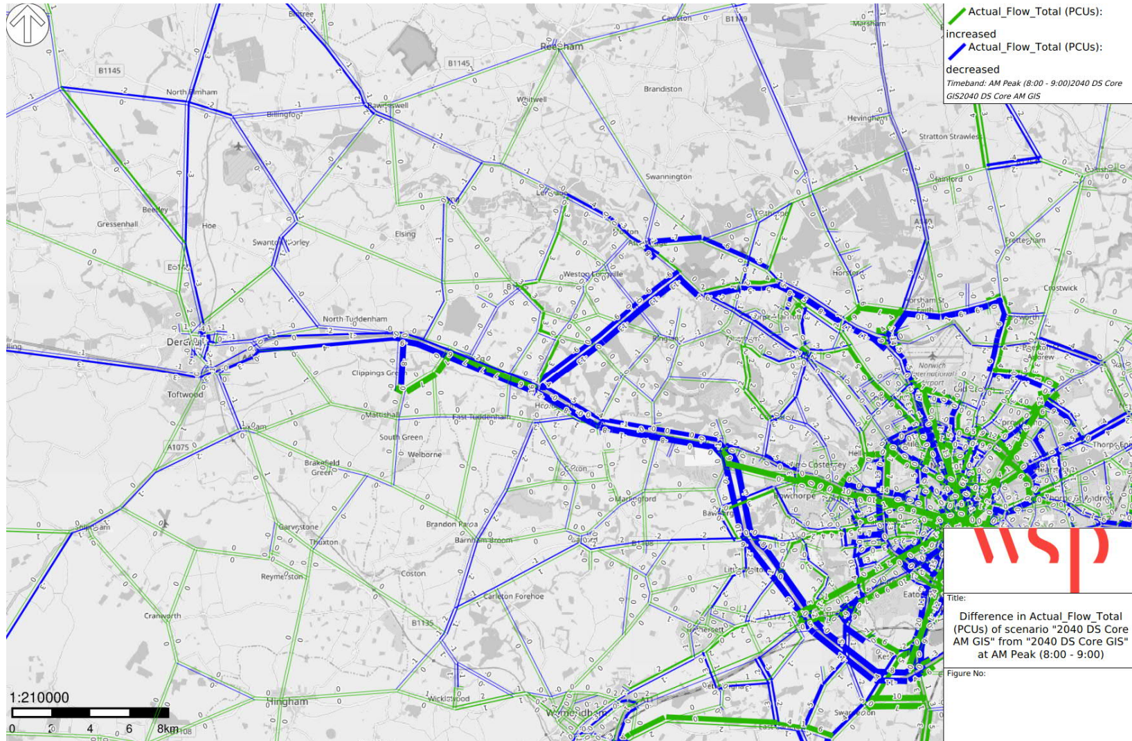
Figure 12-4: 2040 Core Growth DS scenario versus 2040 Core Growth Sensitivity DS scenario, Actual Flow Difference, in pcu's - AM peak
