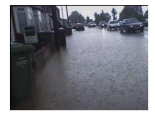
Causes - Run-off from rainfall was concentrated along overland flowpaths on which the affected properties are positioned. Surface run-off from rainfall made its way onto the highway and flowed along the road network and onto the accesses of affected properties that were situated lower than
