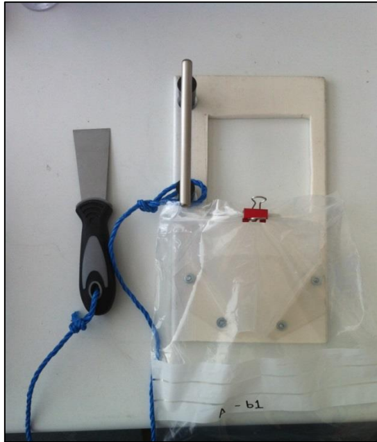
Figure 4. APEM's wall scrape sampling device
