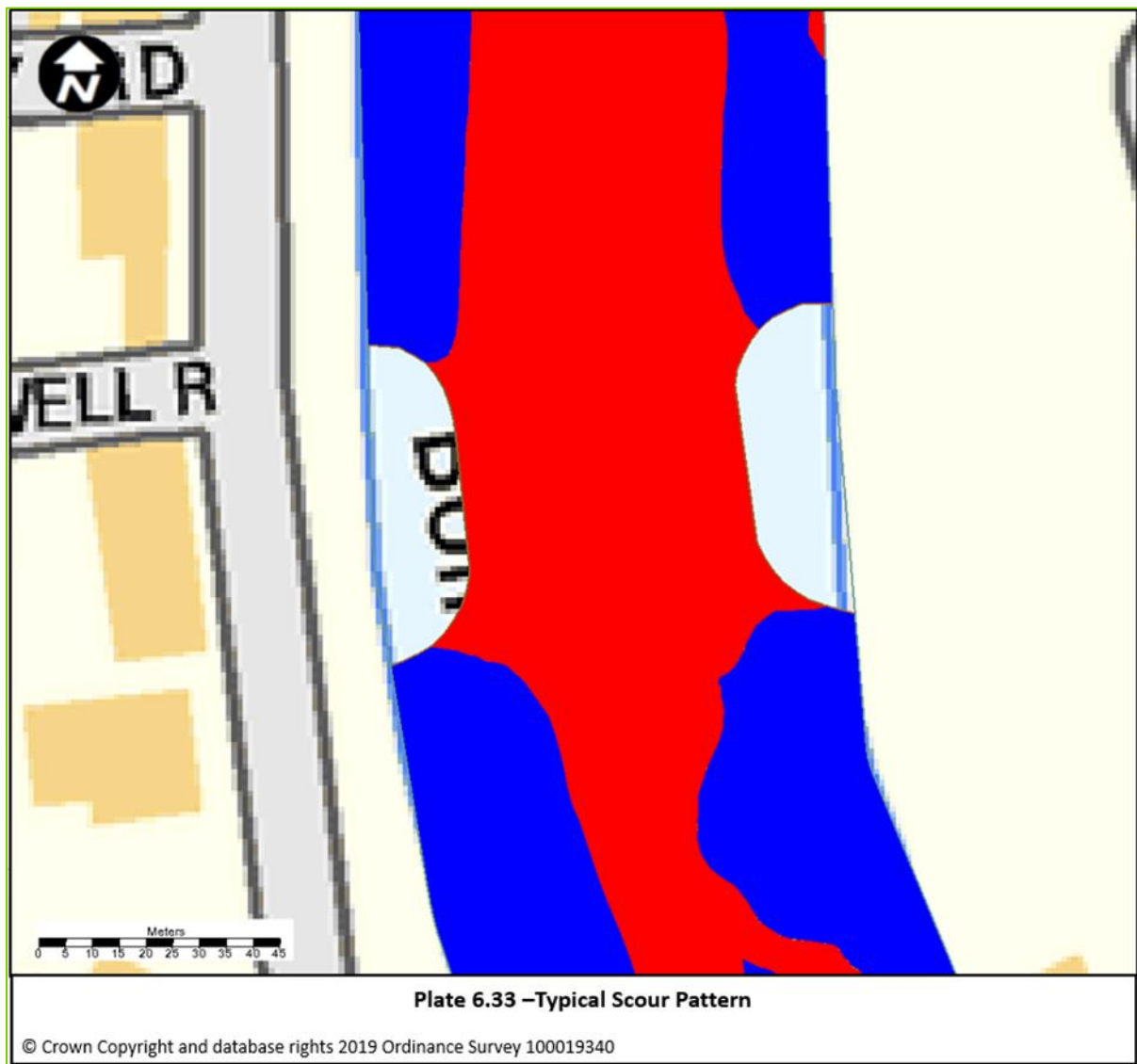
Plate 6-33: Typical Scour Pattern
