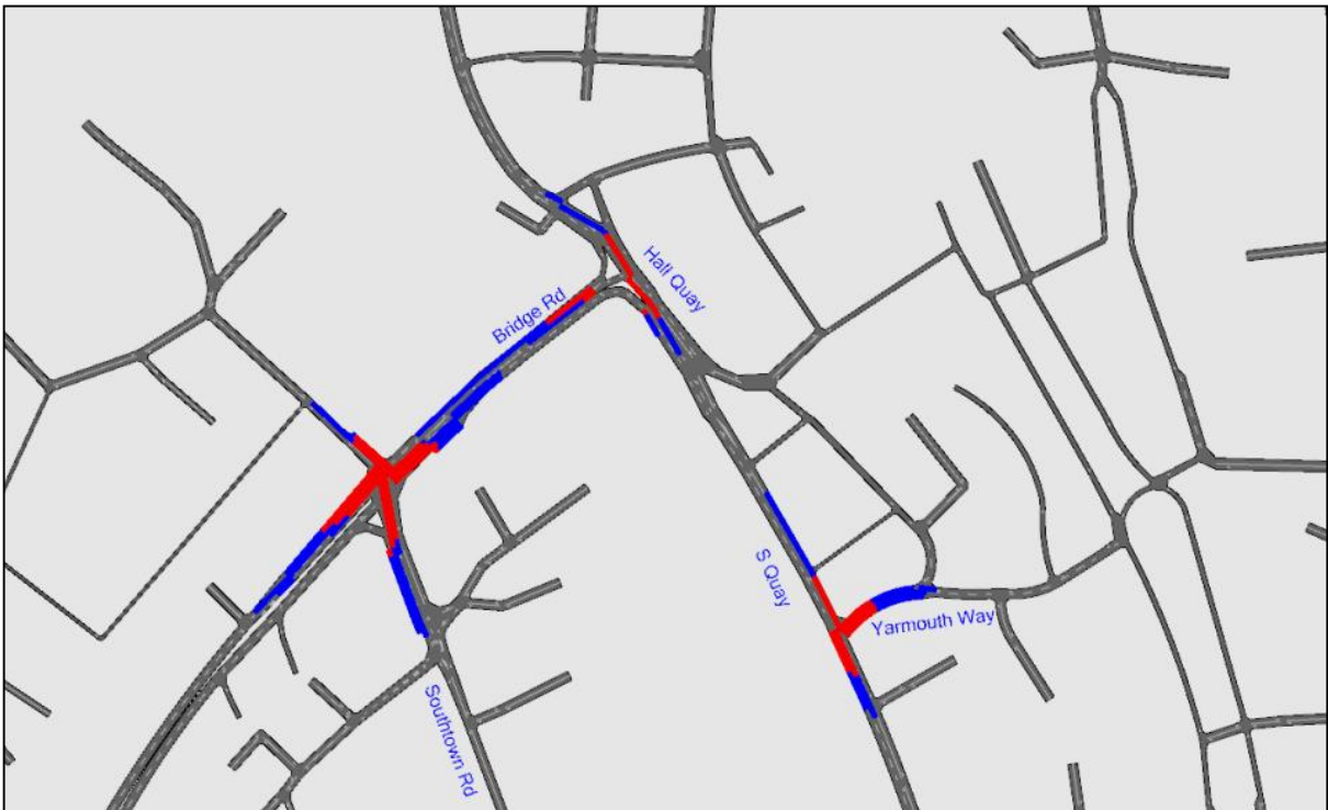
Plate 7-16: Queuing at Junctions near Haven Bridge, 2023 PM (DS)
