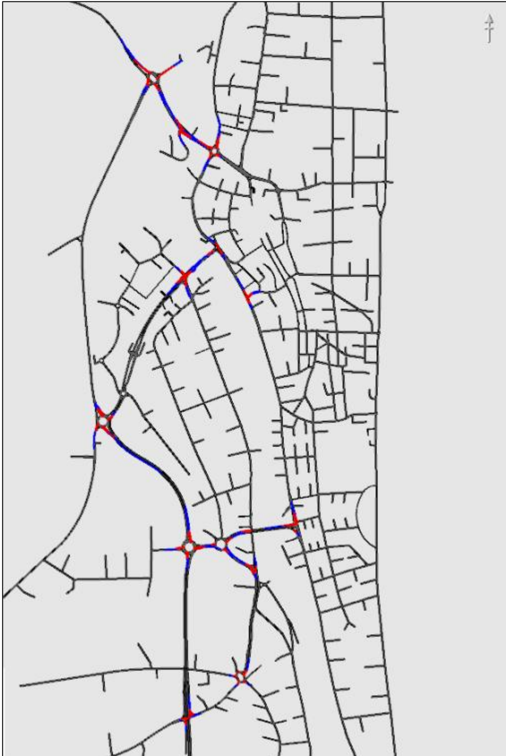
Plate 7-10: PM Peak Queue Lengths at Critical Junctions (DS) - with Scheme
