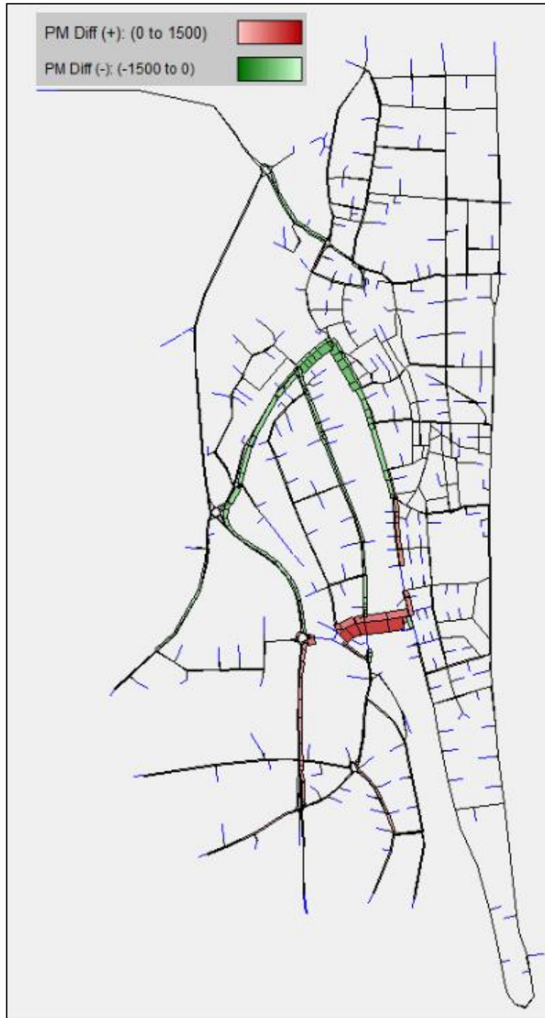
Plate 7-5: Changes in Traffic Flow due to the Scheme (2023 PM peak 1630-1730)
