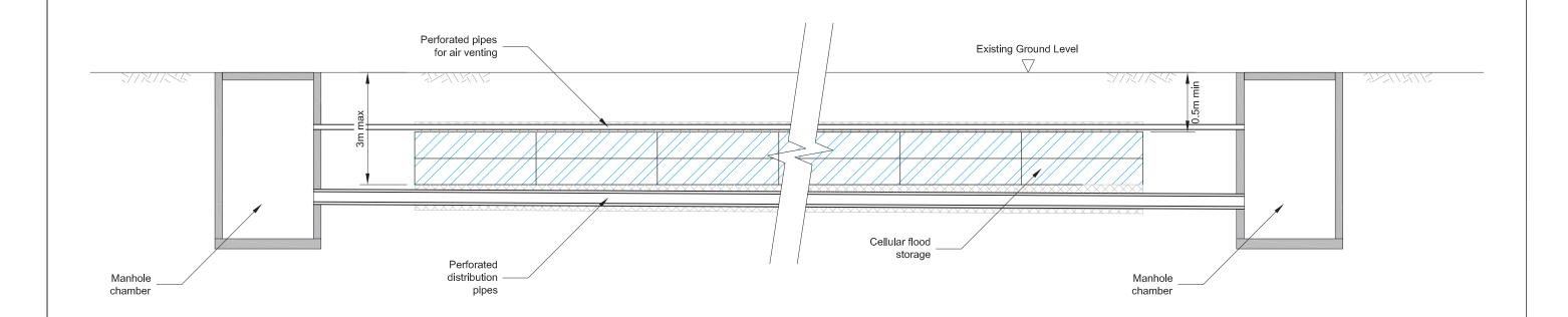
Typical Underground Flood Storage Cross Section
