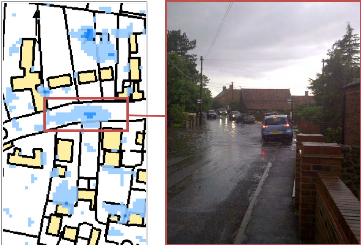
Figure 2-9 Validation of model outputs with local information (Station Road, Heacham)
