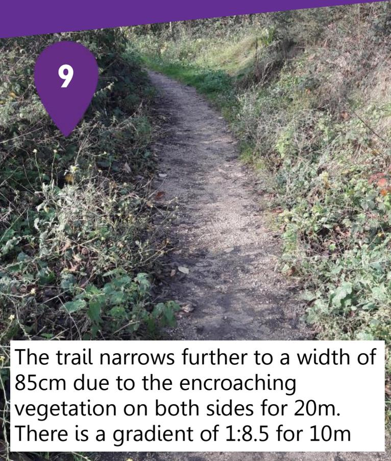
The trail narrows further to a width of 85cm due to the encroaching vegetation on both sides for 20m. There is a gradient of 1:8.5 for 10m
